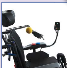
Chin control with a "foam ball" on a mechanical or electrical, retractable arm
