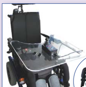
Central control on special retractable shelf (the occupational therapist will determine the joystick position).
