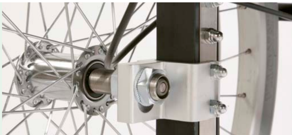
Rear wheels with quick-release axles
