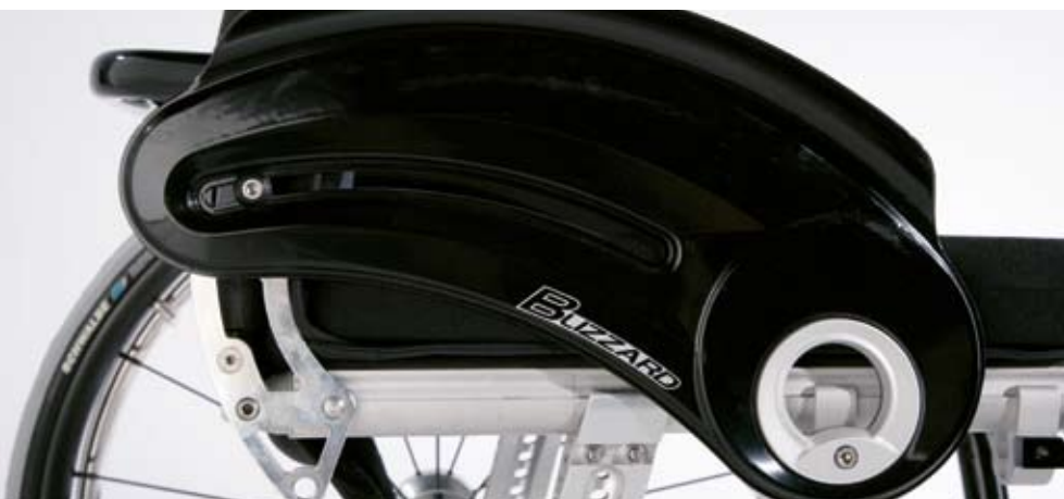
Clothing protector side panel with eccentric disc for fine adjustment
